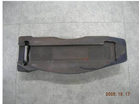
Fig. 4. New model brake pad and brake lining head for VVVF railroad stock (SBK14 ; density : 2.18 g/cm 3 , area : 400 cm 2 , and thickness : 35 mm).
