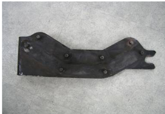
Fig. 3. Old model brake pad and brake lining head for chopper railroad stock (DH2004NA ; density : 2.05 g/cm 3 , area : 376 cm 2 , and thickness : 30 mm).
