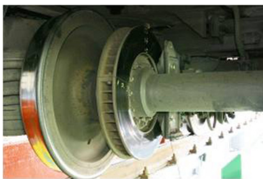
Fig. 9. Modal test of disc assembled body at Gunja depot.
