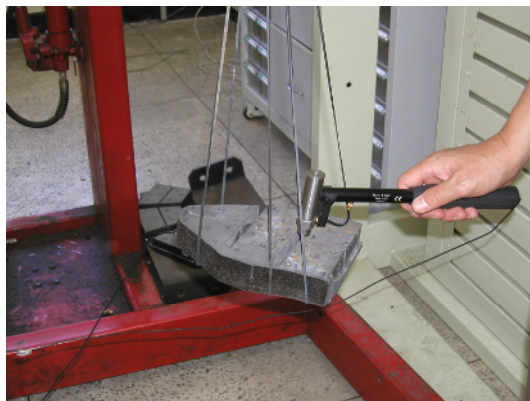
Fig. 8. Modal test of lining pad for VVVF type at SNUT.
